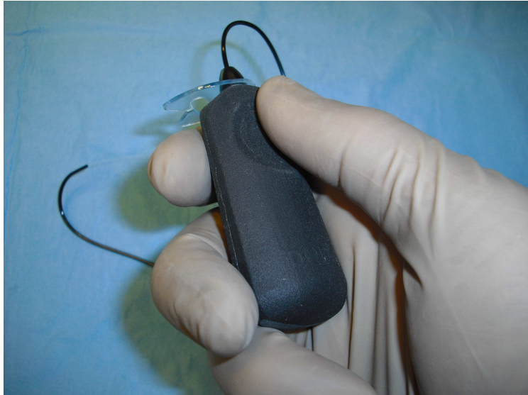
Fig. 39 pressing at sensor of the sterile case for illuminating the fiber
