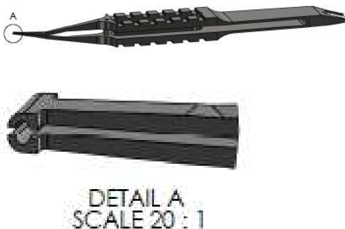
Fig. 42 New glaucoma forceps with special designed tip for better control of glaucoma surgery fibers and atraumatic grasp of ocular tissue, parabolic marker at distal end for marking the superficial scleral flap
